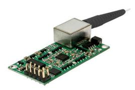
Agiltron offers Fiber Optic MEMS Tunable Filters with central wavelengths of 1060nm, 1310nm, 1550nm, and 2000nm. It is tunable continuously over a spectral range of up to 80nm at a speed of about 80ms. The wavelength tuning is actuated by driving a rotating MEMS mirror that is optically coupled with a grating and a dual fiber collimator. It is conveniently controlled with a user-friendly GUI and USB or RS232 and I2C control interfaces.
